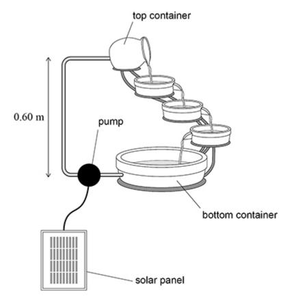
Solar energy is incident on the solar panel at a rate of  $1.5\ W.$  Water from the bottom container is continually pumped through a vertical height of  $0.60\ m$  to the top container.
